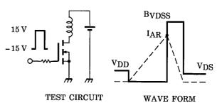
$$\begin{aligned} R_G &= 25~\Omega \\ V_{DD} &= 90~V,~L = 7.35~mH \end{aligned} \quad E_{AS} &= \frac{1}{2} \cdot L \cdot I^2 \cdot \left( \frac{BVDSS}{BVDSS - VDD} \right) \end{aligned}$$
